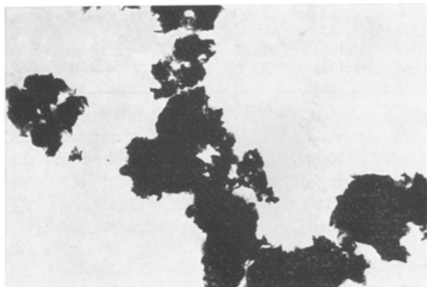
Fig. 5. Electron micrographs of a sample of synthetic montmorillonite after heating at 800^\circ\text{C} ; magnification 7000\times
